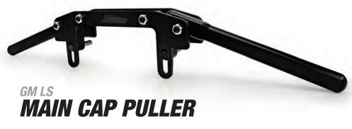
The LS Engine Main Cap Puller is specifically designed to fit LS engines. This sturdy tool makes the job of removing the doweled main caps quick, safe and easy. In one smooth motion, caps are removed and held tightly so they don't fall and become damaged – no prying, hammering or damaging dowels required.
